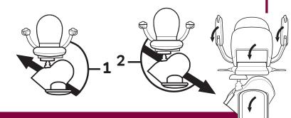
REMINDER - THERE IS A 2 SECOND DELAY ONCE THE TOGGLE OR REMOTE IS PRESSED BEFORE THE LIFT STARTS TO MOVE.
